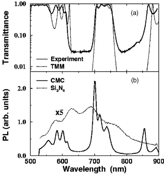
Fig. 2. (a) Comparison of the measured (solid line) and calculated (dotted line) transmission through the  $\text{Si}_3\text{N}_4/\text{SiO}_2$  coupled micro-cavity structure. (b) Measured photoluminescence spectrum of the CMC structure. The  $5\times$  magnified thin curve denotes the PL spectrum of single  $\text{Si}_3\text{N}_4$  layer.
