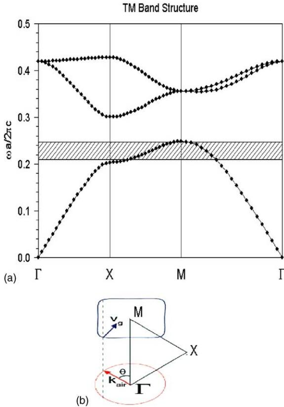
Fig. 8. (a) TM polarized band diagram of the PC. Negative refractive region is shaded. (b) Frequency contours of air (bottom) and PC (top) at  $\omega a/2\pi c = 0.2189$  ( $f = 13.698$  GHz).  $\theta$  denotes the incidence angle from air to PC.
