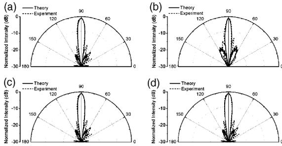
Fig. 7. Measured (dashed curves) and simulated (solid curves) far field patterns at the upper band edge frequency of 13.21 GHz for different lateral lengths of the PC (a)  $32 \times 16$ , (b)  $28 \times 16$ , (c)  $24 \times 16$ , and (d)  $20 \times 16$  layers.
