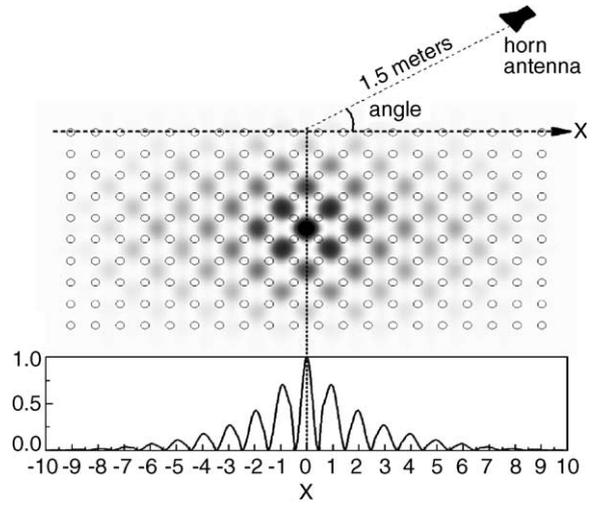
Fig. 5. (a) Experiment setup for a 2D  $20 \times 10$  square array PC. The electric field intensity distribution of a source located at the center and operating at the second band edge frequency. Note the field is localized in between the dielectric rods (air). (b) Lateral distribution of the electric field intensity along the upper surface of the PC.
