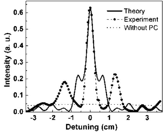
Fig. 11. Focusing: Measured power distribution (dots) and calculated average intensity (solid curve) at the image plane. Full width at half maximum of the measured image is  $\sim 0.21\lambda$ . Spatial power distribution without PC is also shown (dotted thin line).
